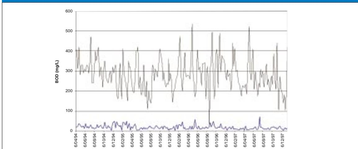
Figure 2.4. Suspended solids in the untreated sewage (higher line) and in the treated effluent (lower line) for ETP.
