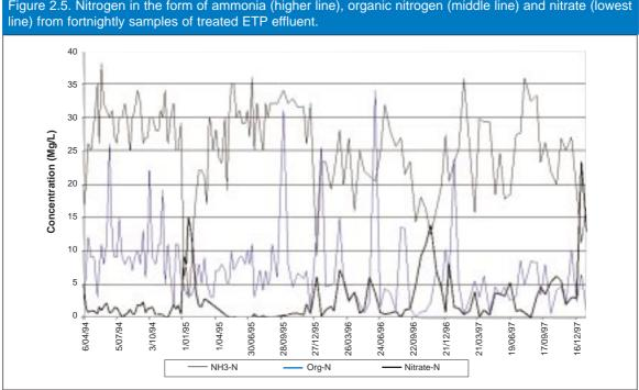
Figure 2.5. Nitrogen in the form of ammonia (higher line), organic nitrogen (middle line) and nitrate (lowest
