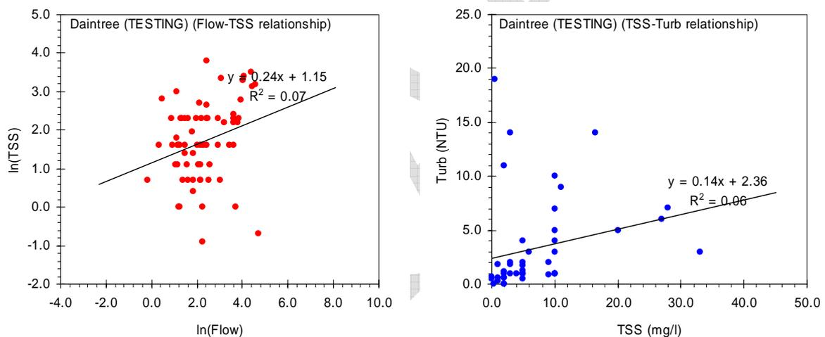
Figure 3.2: Example of scatter plots of  $\ln(\text{flow})$ – $\ln(\text{TSS})$  and TSS-turbidity relationships generated by module/macro M3\_XYPLOT
