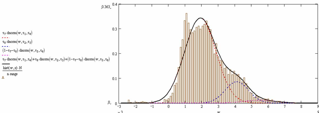
**Figure 2.1: Example of flow regime comprising a mixture of log-normal distribution of base flow (red dotted), wet flow (blue dotted) and storm flow (pink dotted)**
